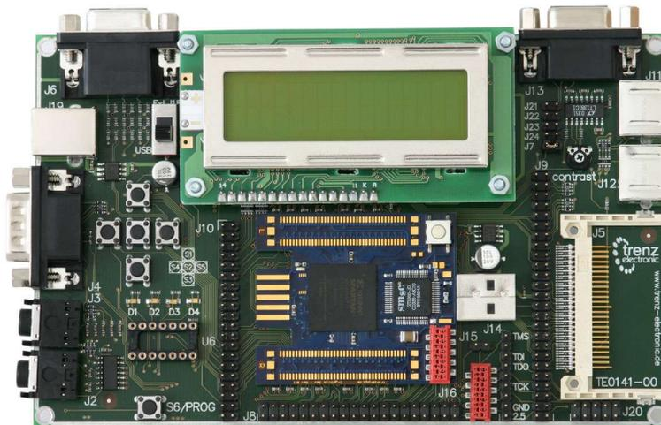
**Figure 1: Baseboard with Micromodule**
