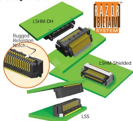
Razor Beam™ interconnects are available in a variety of stack heights from 5mm - 12mm, and the LSEM Series will be available in both
