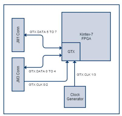
Figure 4: GTX Transceiver block diagram.
