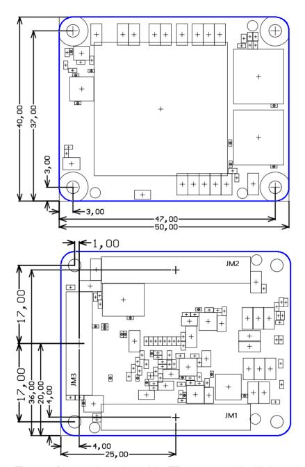
Figure 7: Physical dimensions of the TE0741-02 module. All dimensions are shown in millimeters.
