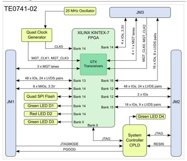
Figure 1: TE0741 Block diagram.
