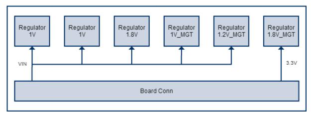
Figure 6: Connections between the on-board DC-DC and LDO regulators.
