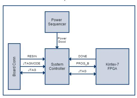
Figure 5: System Controller block diagram.
