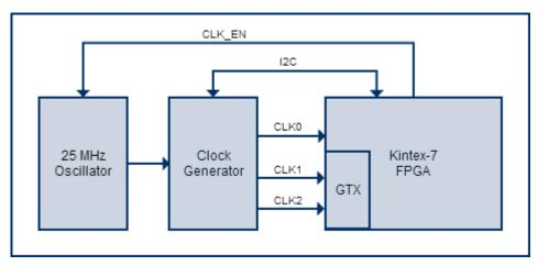
Figure 3: Clock Generator block diagram.
